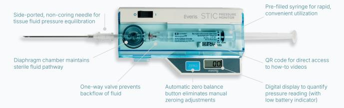
**Quick and Simple Hand-Held Monitor for Accurate Measurement of Compartment Pressure**
